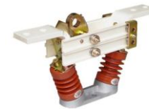
7.2kV 1P 800~1200A Insulating class : 6A(60BIL) Rated Short-time with stand current : 25kA / 1sec Auxiliary contacts : - Hook
